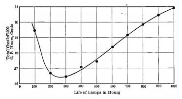
FIG. 156. Curves between useful life and total operating cost of carbon filament incandescent lamps.
